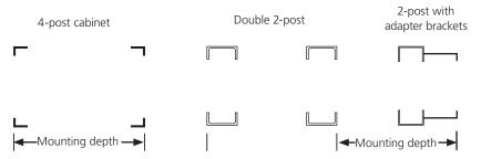
Figure 1. Mounting depth measurements.
